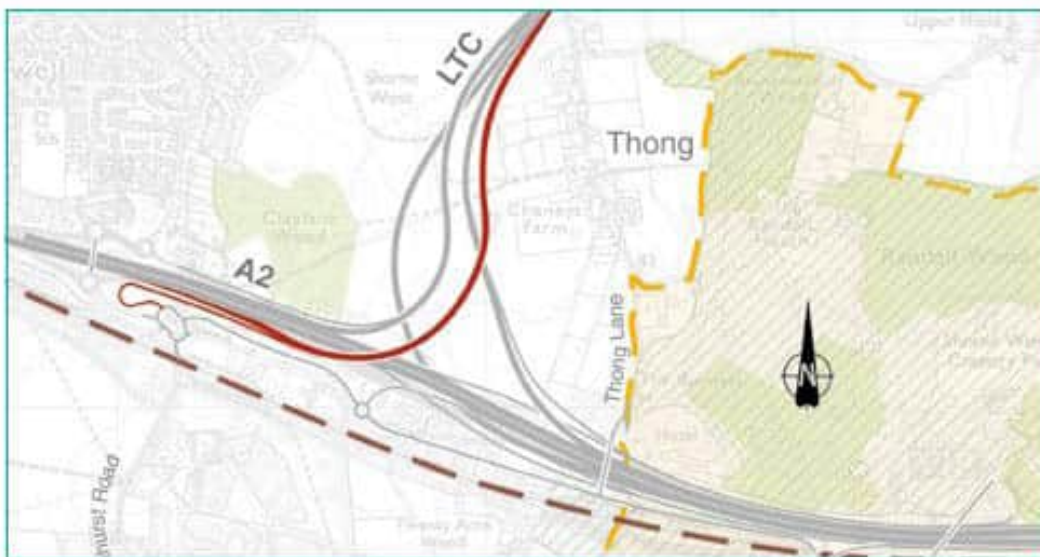
Figure 5 2. Leaving the LTC to join the A2 westbound. Also connects to the Gravesend east junction, where the existing slip road will no longer connect to the A2. The road will pass over the LTC, the M2/A2 westbound to the LTC northbound and the A2 main road
