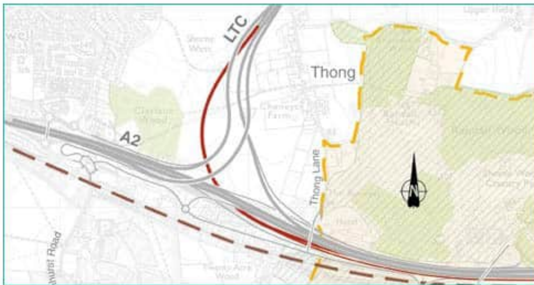
Figure 5.4. Joining the LTC from the M2/A2 westbound. Traffic from the westbound parallel link road will also join here. The road will be in a cutting, passing below the A2 main road and two LTC slip roads
