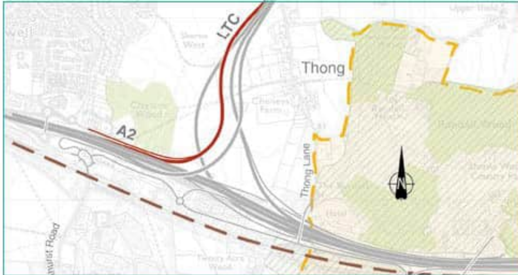
Figure 5.3. Joining the LTC from the A2 eastbound and slip road from the Gravesend east junction. The connection will be elevated on an embankment and will pass over the M2/A2 westbound to the LTC northbound twice to merge on the left
