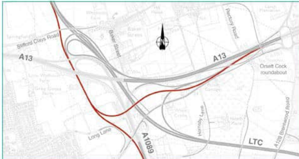
Figure 5 27. Joining the LTC northbound from the A13. Traffic leaving the A1089 northbound also joins this connection. This connection is in a cutting as it leaves the A13 at Orsett Cook. It travels under the realigned Orsett Cook roundabout A13 westbound on slip road, over the A13 westbound to the LTC southbound and the A1089. It is in a cutting to pass under the A13 and Stifford Clays Road and joins the LTC northbound
