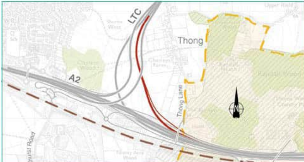
Figure 5 1. Leaving the LTC to join the M2/A2 eastbound. Slip road leaving the LTC southbound divides to connect to both the M2/A2 and the eastbound parallel link road (which leads to local roads). The road passes under the LTC in a cutting before being elevated on an embankment and passing over the A2 eastbound parallel link road
